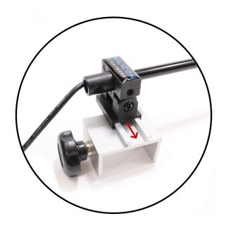
LIGHT ATTACHMENT: On every bracket or clamp you will find an 18mm wide track that pairs with the 2 opposable guide rails found at the base of every light. To attach a light to a bracket or clamp, simply slide the opposable guide rails onto the 18mm track, which will secure the light in place.
