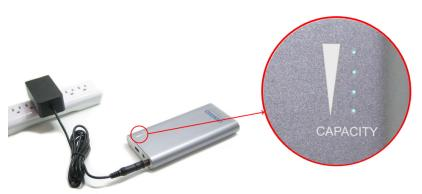
Step 3: Plug the AC Adapter into any standard outlet. The MPC capacity indicator lights will blink while charging and remain fully illuminated when fully charged. Fully charges in approximately 5 hours.
